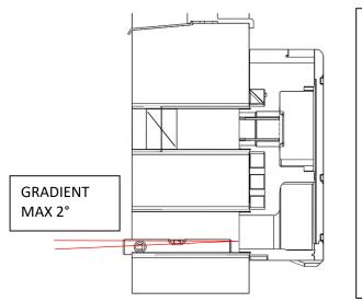
THE FOAM MUST BE APPLIED AROUND THE ENTIRE PIPING LENGTH AND CIRCUMFERENCE – IN CASE OF NON-COMPLIANCE WITH THIS RULE, THERE IS A RISK OF CONDENSATION FORMING ON THE PIPING SURFACE AND FLOW OF THE CONDENSATE INTO THE WALL AND INDOOR AREAS
