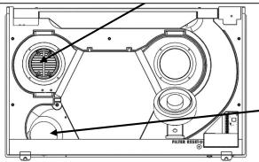
UNIT WITHOUT PREHEATING – VACUUM THE SUPPLY PIPING AND WIPE IT FROM INSIDE (BE CAREFUL NOT TO DAMAGE THE DAMPER IN THE PIPING)
