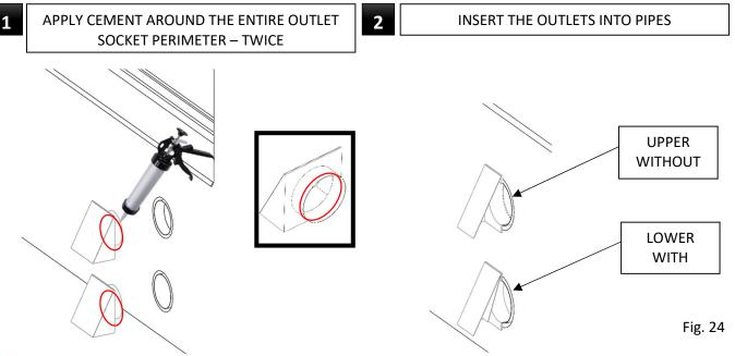
Correct sealing between the damper socket and piping ensures correct condensate drainage through the outlet.
