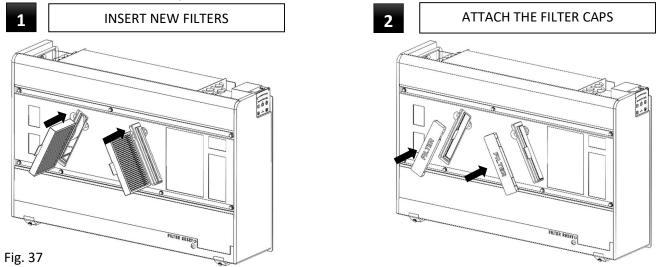
Pay attention to the correct orientation of the caps, they fit only in one position. The FILTER sign must be oriented bottom-up.
